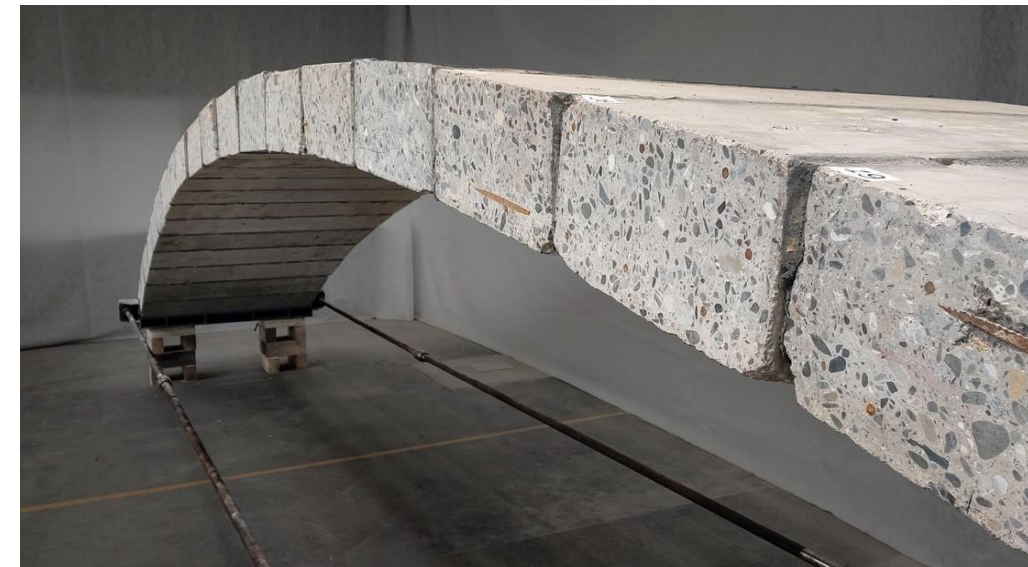
EPFL researchers have built a footbridge prototype using reinforced-concrete blocks from walls of a building being renovated.
